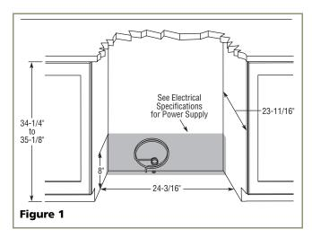
Follow the cut-out drawing in **Figure 1**. The 24-3/16" width allows 1/4" for ease in installation and removal of the unit. 24" is the counter depth in most installations. The unit is 23-11/16" deep including the handle on Black and White models and 23-11/16" deep including the door and *not* the handle on Stainless Steel models (see **Figure 2**).
